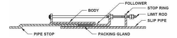
Construction: Similar to details of Style 1 Expansion Joint except that a Stop Ring is welded to the Slip Pipe, and the regular bolts are extended through this ring. A set of double nuts engages the Stop Ring to limit the Slip Pipe from pulling out of the joint.
