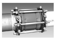
Hand tighten the actuating screws until all wedges are touching the pipes. Continue tightening the screws in an alternating manner until the torque limiting heads twist off. The screws may bottom out during this step.
