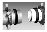
Place the end rings on the pipes with the lip extensions toward the pipe ends. For 14 inch and above Ductile Iron pipe the restraint ring will be the Series 1100 MEGALUG<sup>®</sup> and for C905 PVC 14 inch and above the restraint ring will be the Series 2000PV MEGALUG. Lubricate and install the Standard Mechanical Joint Gasket.
