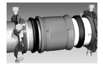
Center the sleeve body over the ends of the pipes while maintaining a 1/2" to 1" gap between the pipe ends. Slide the gaskets and end rings toward the sleeve body.
