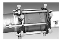
4. Install the threaded rods and hand tighten the nuts on each end. Gradually tighten the nuts in an alternating manner until the proper torque value has been reached, while maintaining the same distance between the rings and the ends of the body at all points around the rings. For 14 inch through 24 inch torque to 75-90 ft.-lbs., for 30 and 36 torque to 120-150 ft.-lbs.
