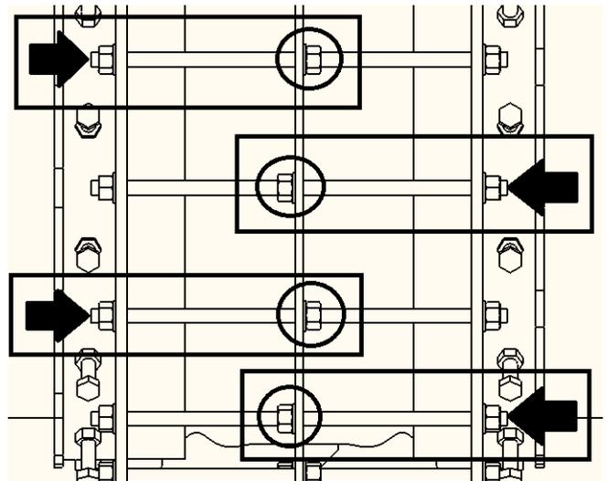
17. Drive all radial gripper bolts of both glands inwards so that they just touch the pipe. Apply no amount of torque to do this. No special pattern is required to do this.
