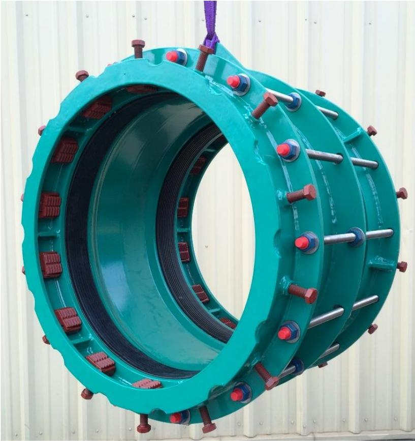
5. Sling the coupling, lift it off of the pallet and remove all wood dunnage from between the glands and the barrel ring.
